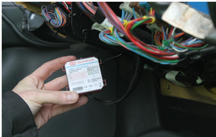
NO x aftertreatment system defeat device
