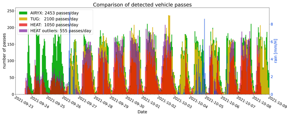
Figure 35. Comparison of passages per day for the different instruments. The HEAT/EDAR instrument configuration in Milan which was not allowing measurement during rain events.
