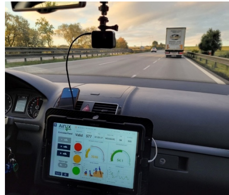
Figure 120: The tablet is used to display real-time data and is connected to the ICAD instrument via WIFI.
