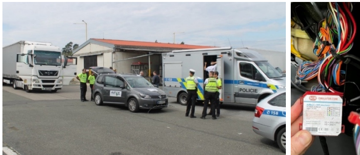
Figure 124: High NO x emitter inspection of HDVs by Czech police (left); emulator that was found during inspection of high NO x emitters identified by the Plume Chasing method (right).
