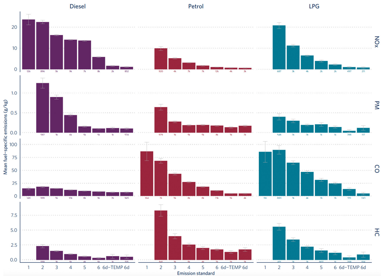
Figure 81. Fuel-specific emissions from diesel, petrol, and LPG passenger cars after filtering out for ambient temperature below 5°C for PM and HC. Only results from 100 or more measurements are presented.
