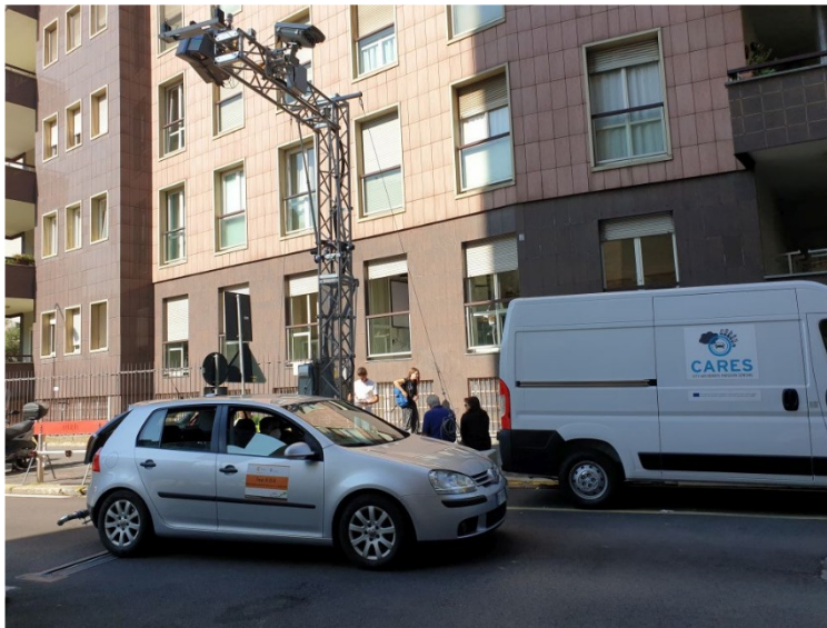
Figure 2. PEMS-equipped high emitting vehicle passing by the overhead remote-sensing unit and point sampling in Madre Cabrini, Milan.
