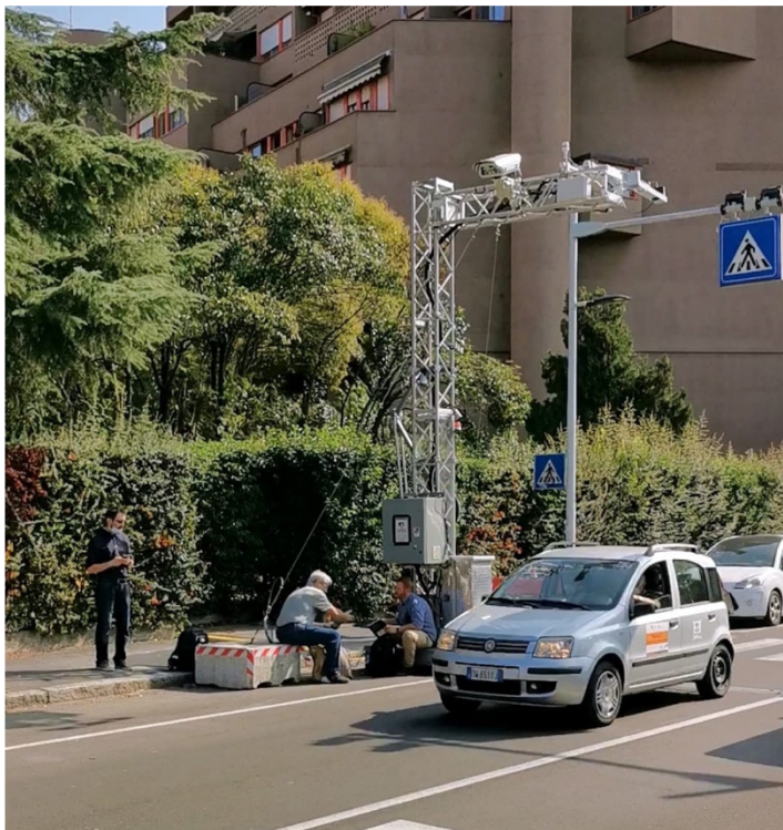
Figure 4. PEMS-equipped bi-fuel vehicle passing by the overhead remote-sensing unit in via Cilea, Milan.
