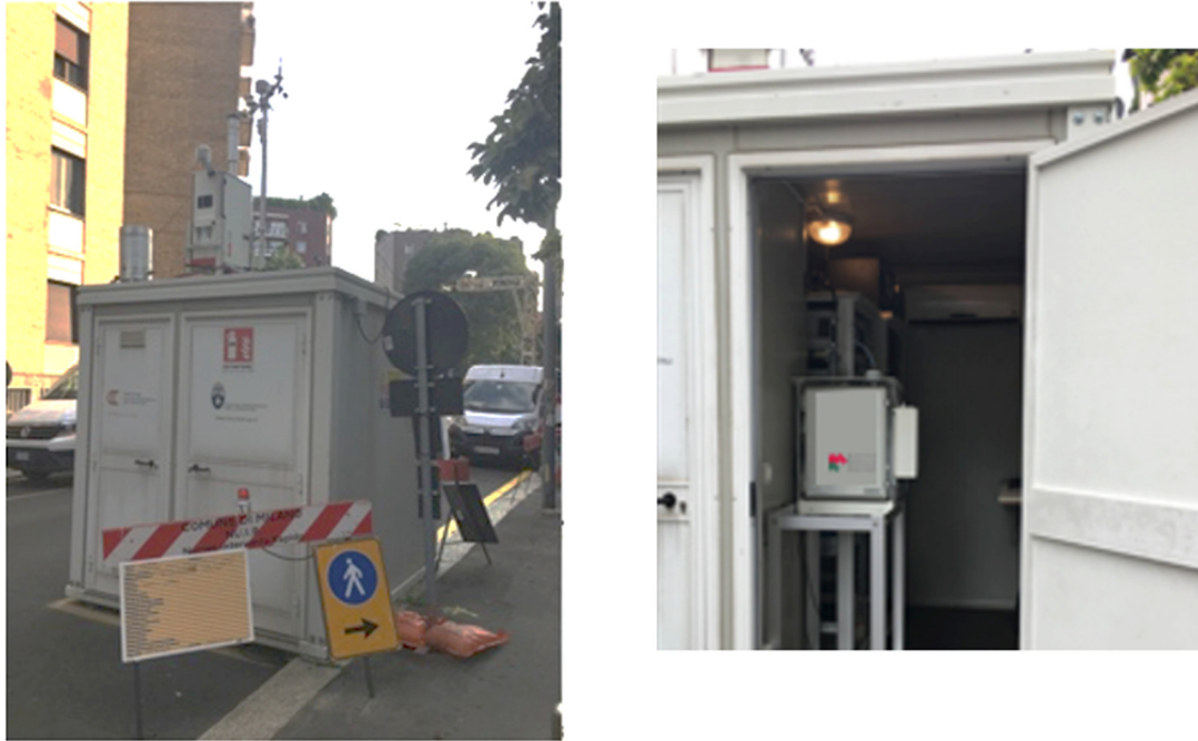
Figure 44. Reference cabin (left) and advanced AQ sensors compact station (right) for monitoring airborne concentrations, and weather conditions in via Madre Cabrini, Milan (Italy).
