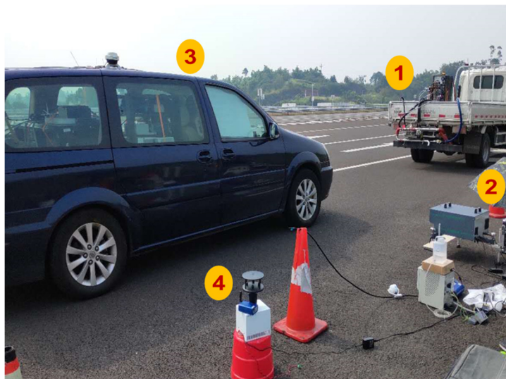
Figure 4 Roadside micro station measurements (marked as 4) in Yancheng, 2020 (1: PEMS, 2: Remote sensing, 3: Plume chasing, 4: Roadside micro station)
